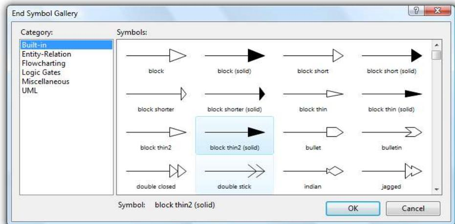
The dialog box displays the installed end symbols. The highlighted box indicates the selected symbol. At the left is a list of categories.
